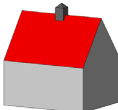
LoD2: simplified building installation
